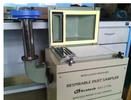
Figure 1. Indian Patent filed for Multiple Slit Nozzle-based High Volume PM 2.5 Impactor Assembly developed in this study
