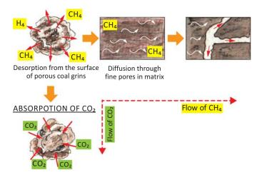
A schematic illustration suggesting the micro-mechanics and processes during  $CO_2$  injection mediated enhanced  $CH_4$  recovery. [Mukherjee & Misra, Earth Science Reviews, 2018]
