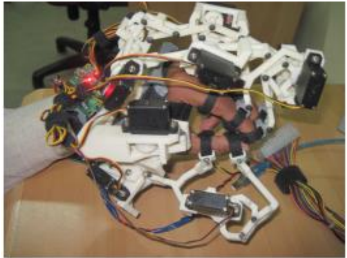
Figure #8: Three Finger Hand Exoskeleton for Translation of a slender object. [Shyam, et al. 2014]
