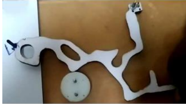
Figure #5: Synthesis of C^0 Path-Generating Contact-Aided Compliant Mechanisms Using the Material Mask Overlay Method. [Prabhat Kumar, et Al. 2016]
